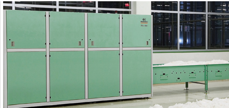
B14 & B15 (+B18) Processed material Cotton, man-made fibers and blends up to 600 kg/h the B14, 300 kg/h the B15, depending on the processed fibers
