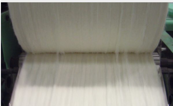
Standard lap winders: irregularity of the superimposed cotton layers
